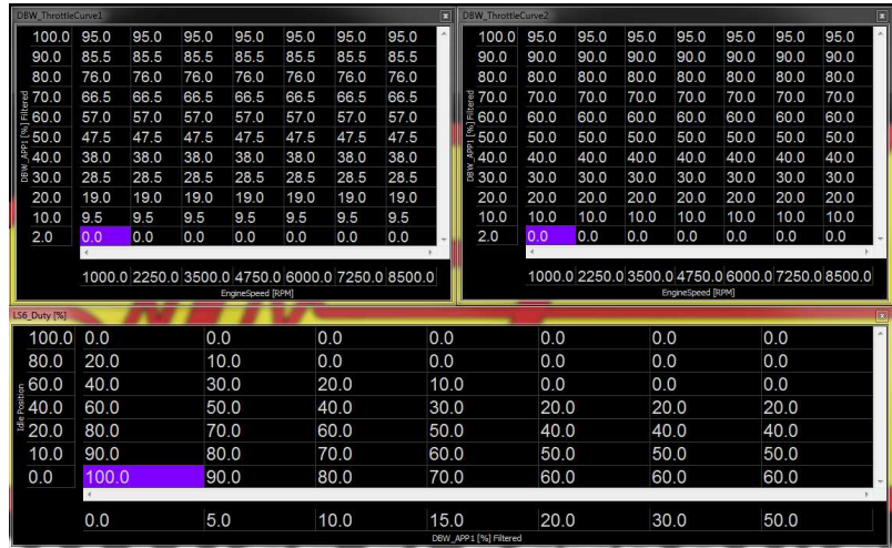
When accelerator pedal is pressed, idle valve sends more airflow into engine. Airflow increases when LS5_Duty is set to low values.
