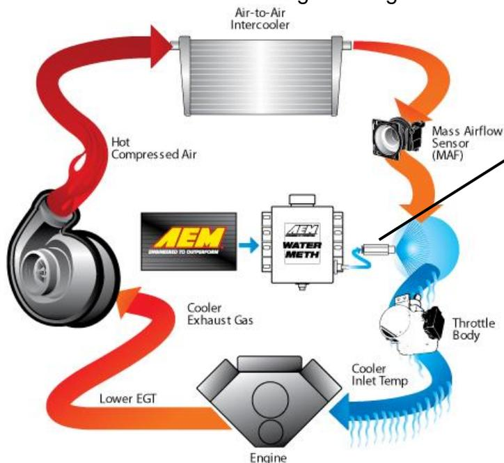
Nozzle installed before the throttle plate, after the MAF and any intercoolers.
