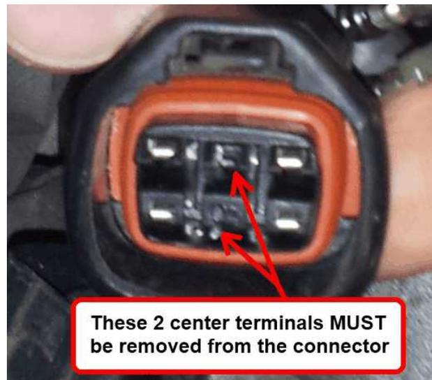
Step 1: Disconnect connector from IACV housing and gently remove the retainer from the connector.
