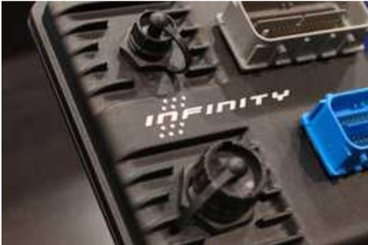
The Infinity ECU includes high quality weatherproof bulkhead USB communications. The smaller connector is for PC communications. The larger connector is for logging to a USB stick. Plug one end of a standard USB extension cable (included) into the smaller ECU connector and the other end into an open USB port on the PC. Communication is possible only when the ECU is powered up.
