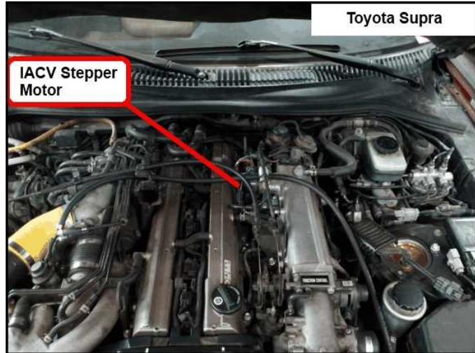
The 2 center pins (Black-Red wires) supply 12V power to the stepper motor in the factory setup, however these pins **MUST BE DISCONNECTED** before powering on the AEM Infinity ECU.
