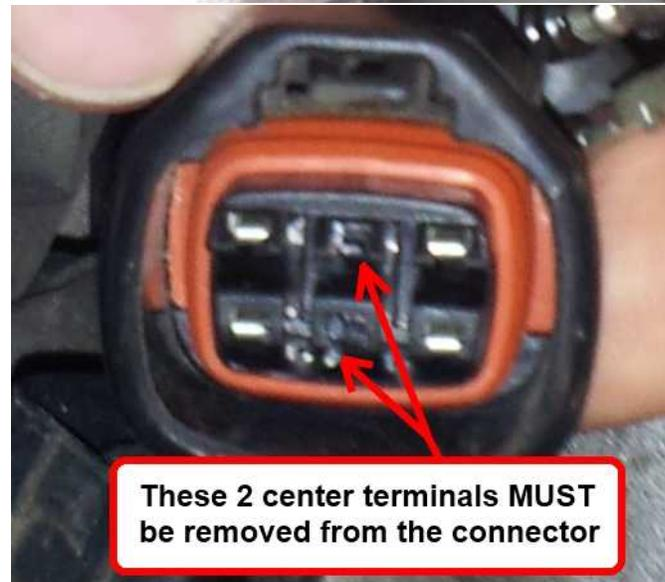
5. Using a small flat-blade screwdriver or pick, carefully remove the terminal lock.
