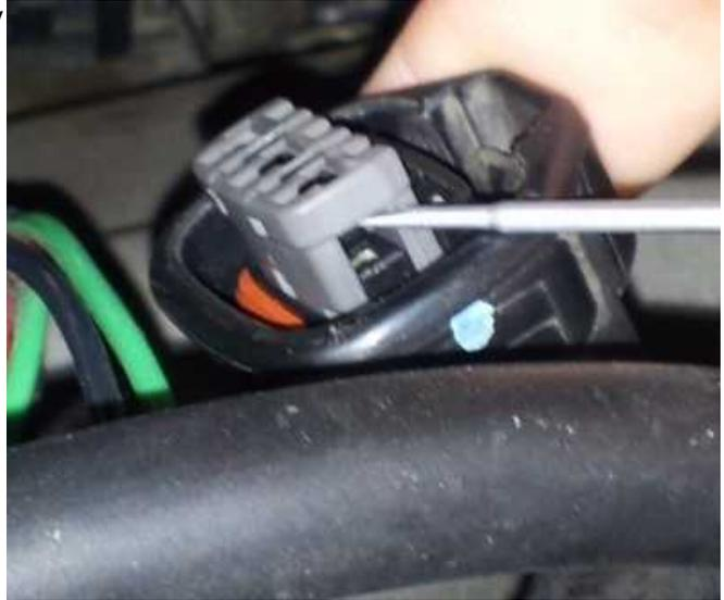
6. Carefully lift the terminal locks while pulling the wires out from the backside of the connector to remove the two center pins.
