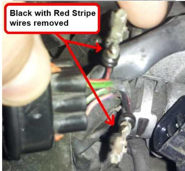
7. Insulate both wires with heat shrink and secure to nearby harness loom.
