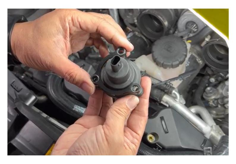
Ensure electrical connectors clip in with a positive click and lock. Once engaged the light grey connector can be pushed in to lock the connector in place. Note: the image below shows correct orientation of the valve and solenoids.
