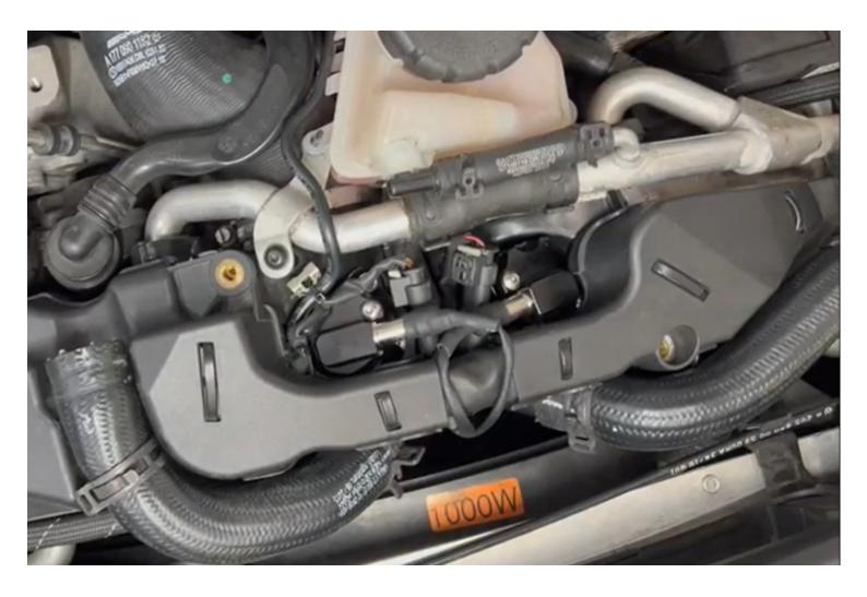
Reinstall intake onto the car. As this car has an aftermarket intake system your specific installation may differ slightly. The recirculation pipes may need to be removed on OEM intakes and some aftermarket intakes to allow for enough room.
