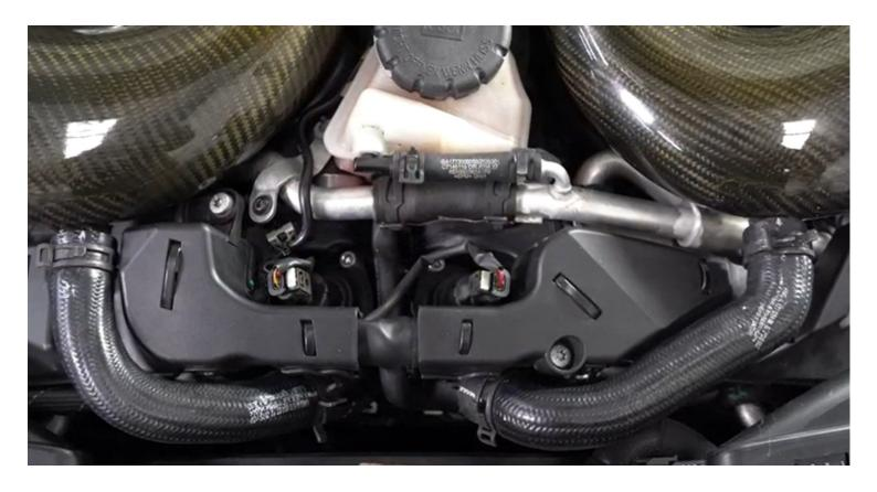
Orientation is important for installation of the Turbosmart EM BOV. A swivel flange is used to allow for easier installation. Once the standard OEM diverter has been removed. Match up the orientation of the valve with orientation of the OEM the swivel flange.
