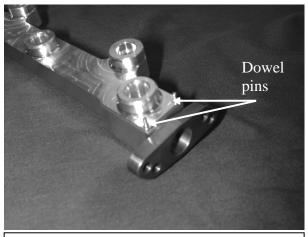
f) *Gently* insert the end adaptor into the fuel rail. Make sure the o-rings stay in place and are not torn. Insert two 1-2061 dowel pins into the dowel pin holes.
