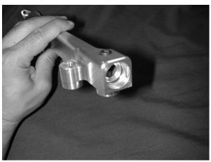
**c)** Insert one 1-3024 o-ring into the inner groove. Make sure the o-ring is evenly seated in the groove.
