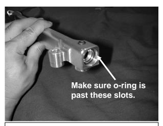
d) Insert another 1-3024 o-ring up against the first shoulder. Make sure the o-ring is seated evenly against the shoulder and is past the slots for the dowel pins.
