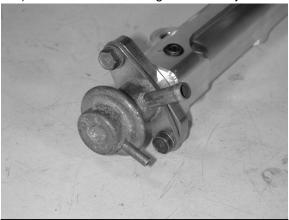
b) Mount the factory fuel pressure regulator to the *AEM* fuel rail using the factory M6 bolts and washers. The *AEM* fuel rail's regulator flange has been designed to be used with both the 1989-1995 and the 1996-1999 model year fuel pressure regulators. Note: Apply a light coat of engine oil to the regulator o-ring before installation.
