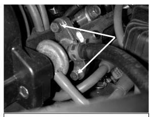
**b)** Remove the two bolts mounting the fuel pressure regulator to the fuel rail. The rail will need to be repositioned before the regulator can be removed due to a lack of clearance with the cam cover.
