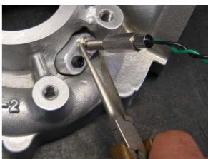
longest end (3 pins, approx. 35.5 in / 900mm long). This end connects to the speed sensor. Connect the harness to the sensor and lay the harness out in the engine bay to begin determining wiring harness routing. See figure 9 below.
