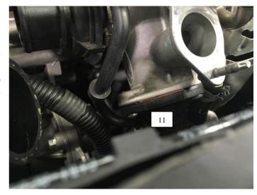
12. Install supplied 6mm plastic blank into OEM BOV signal line and clamp with original spring clamp. This is to ensure there are no leaks.
