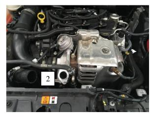
3. Remove turbocharger inlet suction pipe from air filter by undoing the hose clamps and securing nuts.
