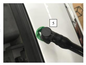
6. Identify this section of the emissions circuit hard-line, there is a 90 degree quick connect fitting with a PCV unit shortly downstream. This quick connect fitting is found directly attached to the intake manifold. This is where the signal for the BOV will be sourced from. Note: This is why it is required to "pull" the emissions line out of the bay slightly to aid in this modification.
