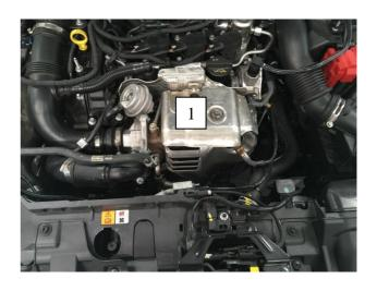
2. Remove charge pipe outlet secured by 2x 10mm nuts and hose clamp.
