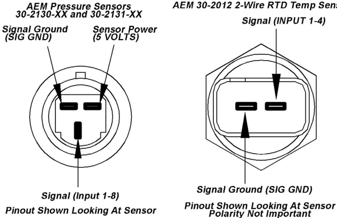
Figure 1. AEM Pressure Sensors(Left) AEM Temp Sensor (Right)
