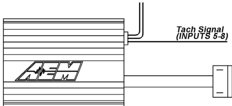
Figure 2. Engine RPM Signal From CDI
