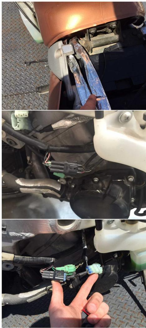
Carefully route the wheel speed connector through the chassis to the Hayabusa wheel speed connector in front of the coolant overflow tank. Unplug the Hayabusa wheel speed connectors and plug them into the Infinity adapter harness. Ensure all cables are securely fastened and routed in a safe manner.
