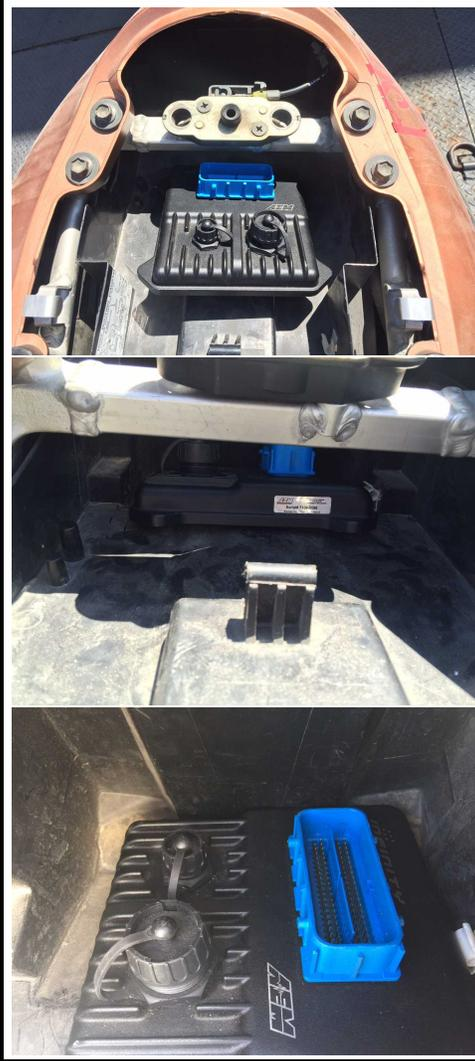
Carefully slide the Infinity into the tail of the Hayabusa as shown. Affix the Infinity to the tail in the orientation shown in pictures 2 and 3 using velcro strips.
