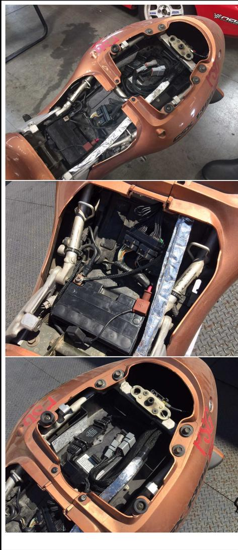
Shown left is what the finished install should look like. Re-connect the battery, re-install the seat, and rear cover.
