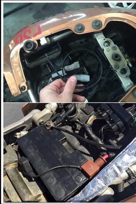
Locate the battery negative ring terminal (NO FUSE ON LEAD) from the coil driver connector and connect to the battery negative terminal.
