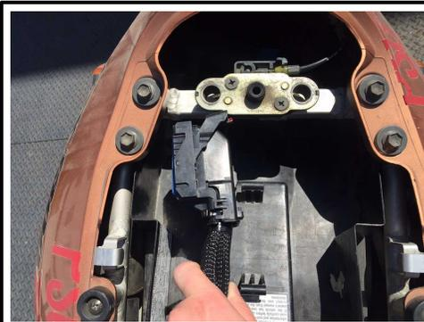
Slide the Infinity Molex 80-pin connector into the Hayabusa tail and plug it into the Infinity.
