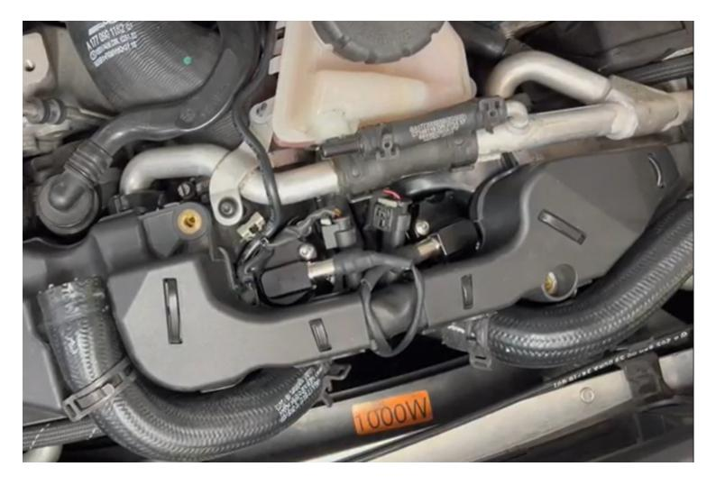
Reinstall intake onto the car. As this car has an aftermarket intake system your specific installation may differ slightly. The recirculation pipes may need to be removed on OEM intakes and some aftermarket intakes to allow for enough room.
