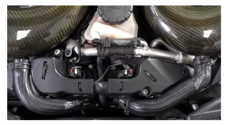
Orientation is important for installation of the Turbosmart EM BPV. A swivel flange is used to allow for easier installation. Once the standard OEM diverter has been removed. Match up the orientation of the valve with orientation of the OEM the swivel flange.
